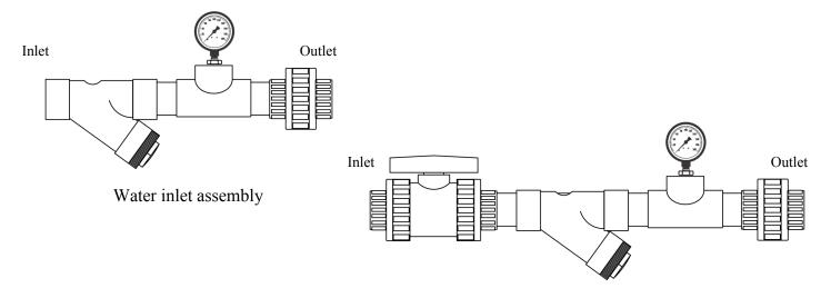
Water inlet assembly with true union ball valve
